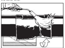
Start heating the sleeve at the side of the leading edge, the side that first comes in contact with the ground forces. Move the torch continuously in a paint brush motion all the way around the sleeve.
