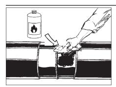
Clean exposed steel and adjacent pipe coating to be covered by DIRAX sleeve. Remove all contaminants such as oil. Use a solvent that contains no grease or oil type materials.
