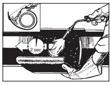
Preheat the inside adhesive layer just next to the closure for a few seconds, and press down on the sleeve end to make it stick to the other end.
