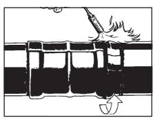
Shrink the leading edge sleeve down by moving the torch all the way around the pipe in a paintbrush motion. Make sure the sleeve has fully shrunk and adhesive flow is evident on both edges.
