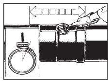
After the DIRAX sleeve has shrunk into the joint area and while it is still hot and soft, run a small hand roller over it to push out any trapped air.
