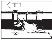
After you have finished heating the side at the leading edge, recover the remainder of the sleeve by heating toward the other end of the sleeve
