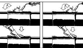
Immediately pat it down firmly with a gloved hand. Continue heating and patting every 10 cm (4") until the whole patch area is finished.
