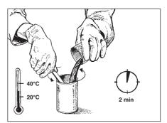
Dose the two component epoxy. Use pre-dosed epoxy kits or use calibrated epoxy pumps.
