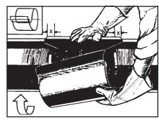
Immediately after application of the epoxy primer, and while the epoxy primer is still wet, loosely wrap the DIRAX sleeve centrally around the welded joint.
